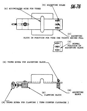
THE ADJUSTING BLOCK ( POSITION B AND C ) CAN BE REVERSED ON THE JIG. WHEN THIS IS DONE THE DRILL BUSHING HOLES WILL BE CENTERED ON A TUBE THAT IS FULL BY AS MUCH AS A THIRTY SECOND.
